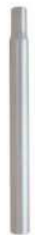
} ZFI2001 MATERIAL: ALLOY 6061 T6 DIAM: \Phi 25 - \Phi 31.8 LENGTH: 250-550mm FINISH: MATT BLACK AND ANODIZED
