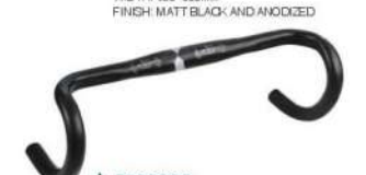
ZFG2022 MATERIAL: ALLOY 6061 T6 DIAM: \Phi 31.8 \Phi 25.4 \Phi 22.2 RISE: 75mm DROP: 145-150mm WIDTH: 380-420mm FINISH: MATT BLACK AND ANODIZED
