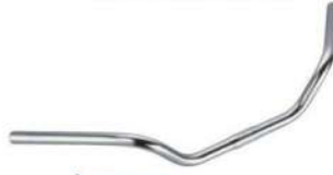
ZFG2014 MATERIAL: ALLOY 6061 T6 DIAM: \Phi 22.2 \Phi 25.4 RISE: 80mm WIDTH: 580-660mm FINISH: MATT BLACK AND ANODIZED
