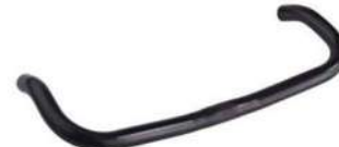
ZFG2009 MATERIAL: ALLOY 6061 T6 DIAM: \Phi 22.2 \Phi 25.4 RISE: 30mm WIDTH: 380-420mm FINISH: MATT BLACK AND ANODIZED
