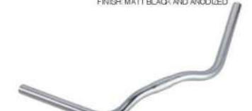
ZFG2008 MATERIAL: ALLOY 6061 T6 DIAM: \Phi 22.2 \Phi 25.4 RISE: 40mm WIDTH: 480-680mm FINISH: MATT BLACK AND ANODIZED
