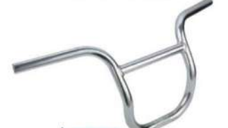
ZFG2019 MATERIAL: ALLOY 6061 T6 DIAM: \Phi 22.2 \Phi 25.4 RISE: 130-250mm WIDTH: 560-660mm FINISH: MATT BLACK AND ANODIZED
