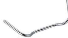
ZFG2013 MATERIAL: ALLOY 6061 T6 DIAM: \Phi 22.2 \Phi 25.4 RISE: 65mm WIDTH: 500-480mm FINISH: MATT BLACK AND ANODIZED
